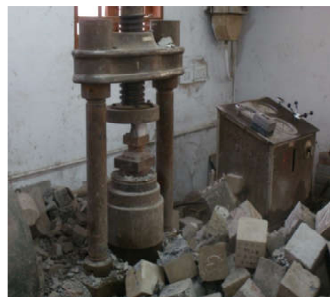
Fig. 9. Cement Mortar cubes being tested under Compression Testing Machine.
